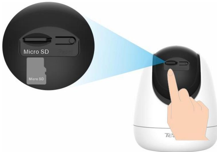
**Step 2** [Log in to TDSEE App](#) to check whether the Micro SD card can be identified normally.
