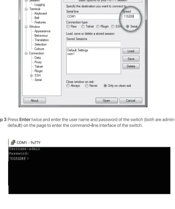
Step 3 Press Enter twice and enter the user name and password of the switch (both are admin by default) on the page to enter the command-line interface of the switch.
